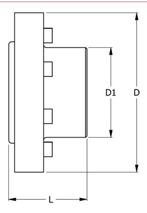
D = 125 D1 = 90 L = 50 Max bore = 55 Torque (N m) = 240
